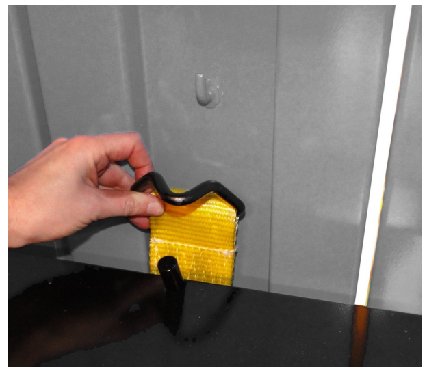
The built in ejection makes it simple to remove the sack or bale from the machine
