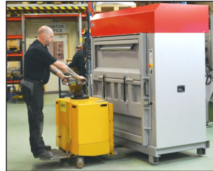
By a pallet truck the machine can be moved from side or front - rationally for placement and simplifies cleaning.
